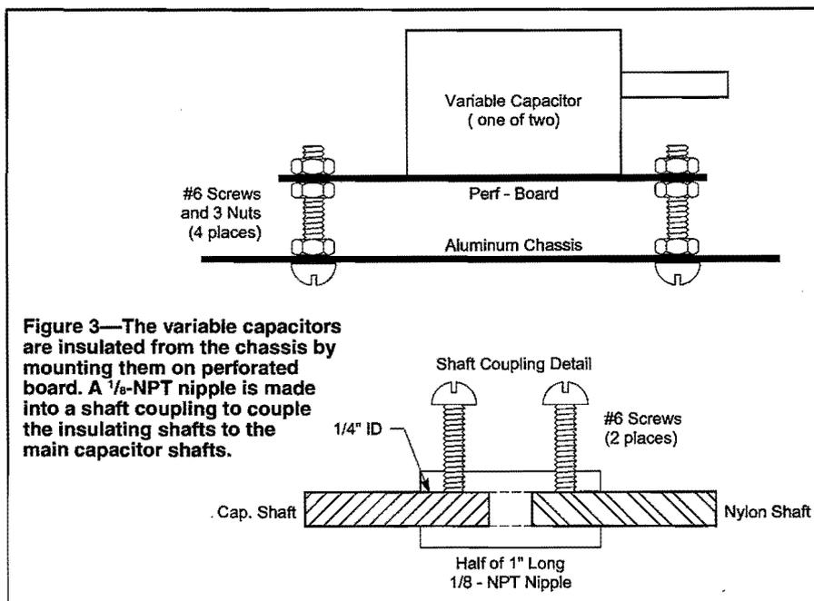
**Figure 3—The variable capacitors are insulated from the chassis by mounting them on perforated board. A 1/8-NPT nipple is made into a shaft coupling to couple the insulating shafts to the main capacitor shafts.**
