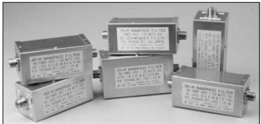
return-loss response. Micrometals specifies a 5% core-permeability tolerance. The resulting L1 and L3 inductance variation is compensated for by squeezing or spreading the turns on the cores until both resonators tune to the same frequency.
