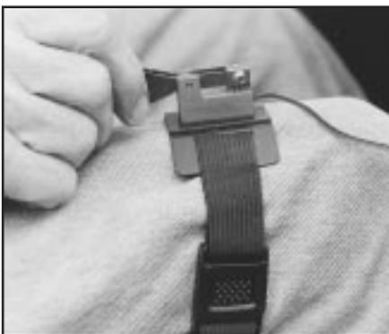
Company's new subminiature keyer paddle, designed for QRP, mobile and backpacking service, that's what!
